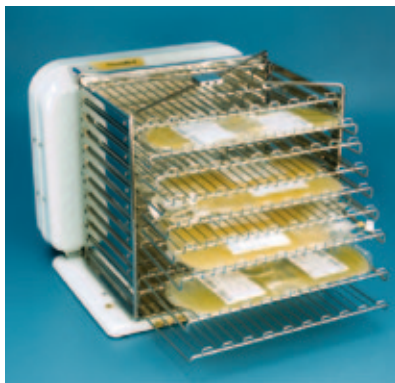
Screen shaped pull-out drawers allow an easy visual inspection and may be removed while the shaker is working
