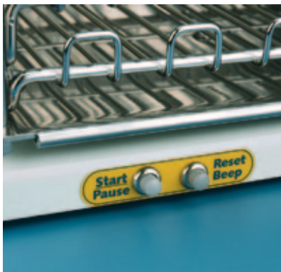
Start/Pause button allows temporary interruption of the movement for loading and unloading the bags on the drawers. To restart the agitation just press the button again.
