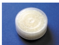
White cartridge indicates humidity damage
